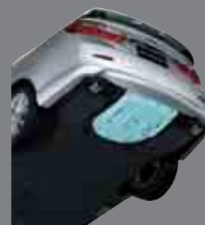
**Aerodynamics:** Among the many measures contributing to the excellent straight-line stability and reduced Cd figures are under covers on the underfloor and aero stabilizing fins to enhance the airflow effect.
