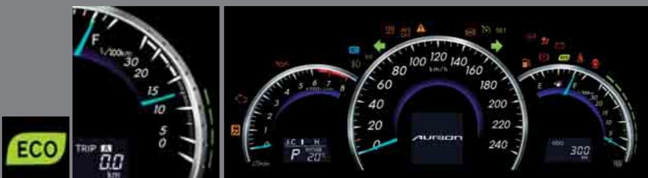
**Meter cluster:** Easy-to-read Optitron meters provide the driver with critical driving information at a glance. To support eco driving, it is equipped with a needle-type average fuel consumption gauge and LED current fuel consumption bars, and an Eco Driving Indicator that illuminates a green lamp to inform the driver when accelerator operation is considerate to the environment.
